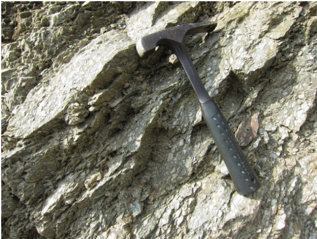
Fig. 10: Outcrop view of weathered Ulleri Augen Gneiss and phyllite near the landslide area
